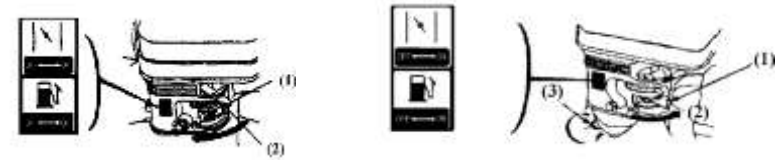
(1) Auto-Throttle (2) Off Position (3) Starter Knob
